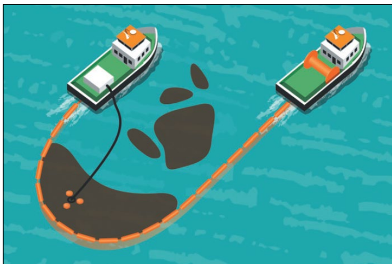
Figure 11-1: 'J' Configuration for Containment & Recovery Operations; 1 x Containment and Recovery Unit (IPIECA-IOPG, 2016a)
