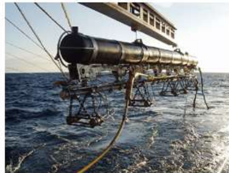
Figure 4-4: Individual compressed air chamber and a sub-array
