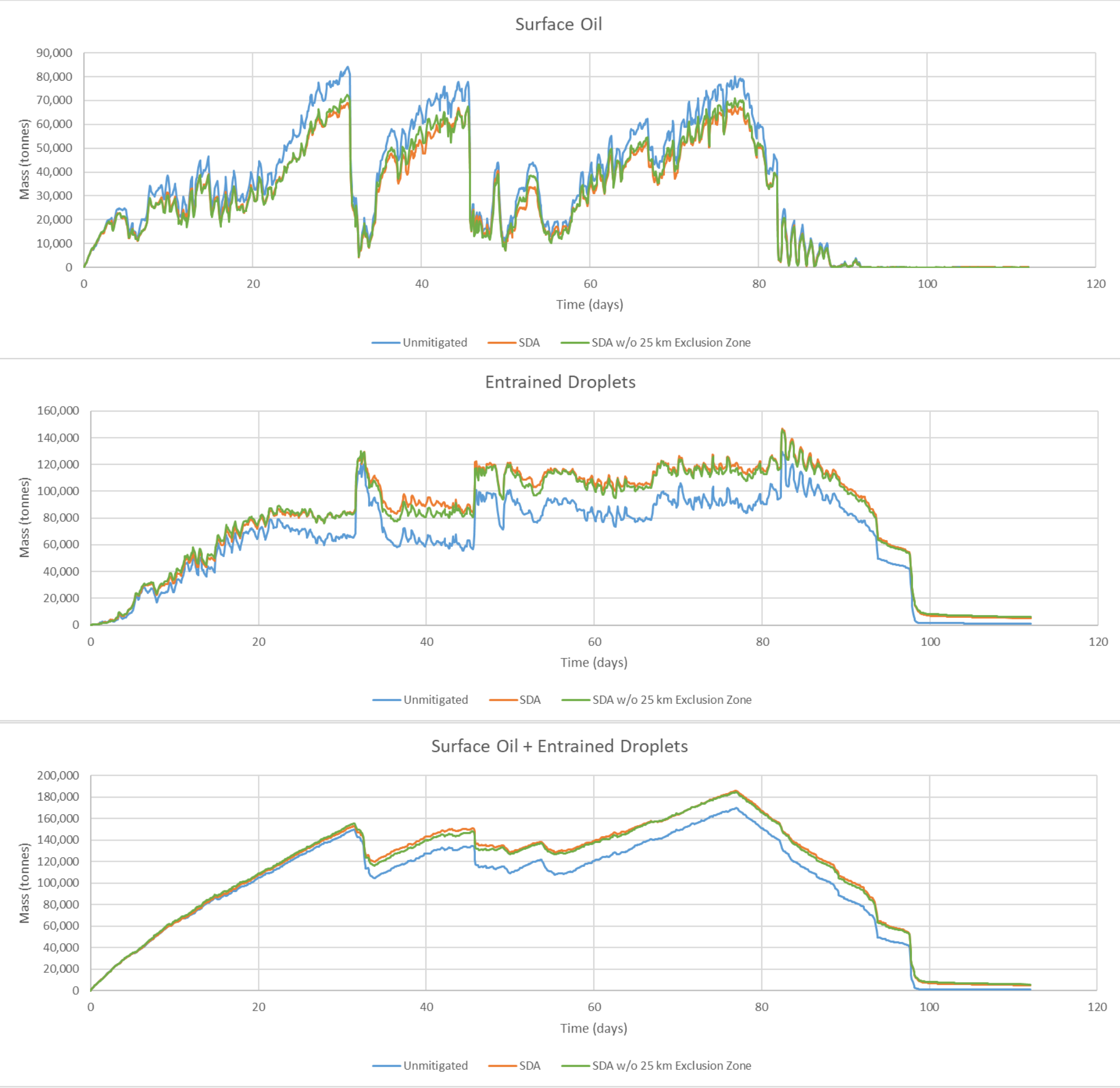
Figure 51 Apus Base Case Surface LOWC Scenario Realisation #31 – Comparison of unmitigated (blue), SDA mitigated (orange) and SDA mitigated without 25km exclusion zone (green) surface oil mass (top panel), entrained droplets (middle panel) and combined surface and entrained mass (bottom panel)
