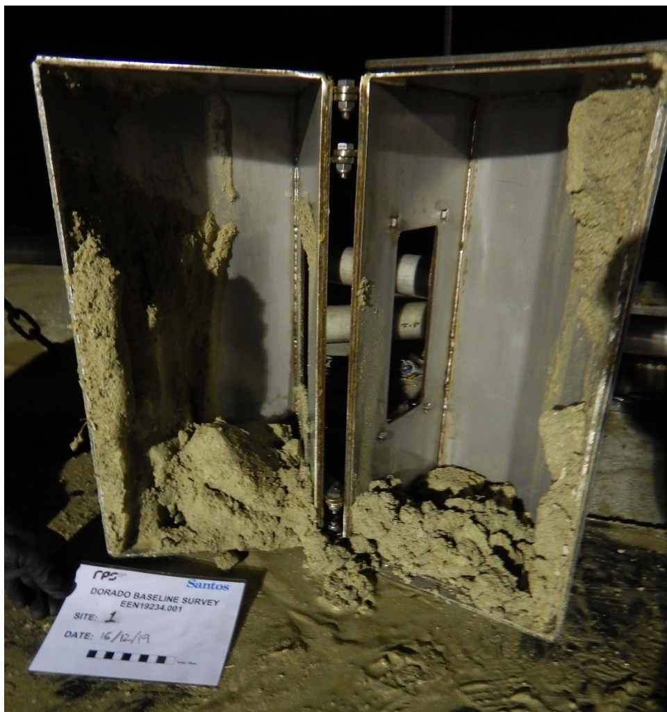
Figure 2-3: van Veen grab (0.25 m 2 ) with infauna sediment sample from Site 1
