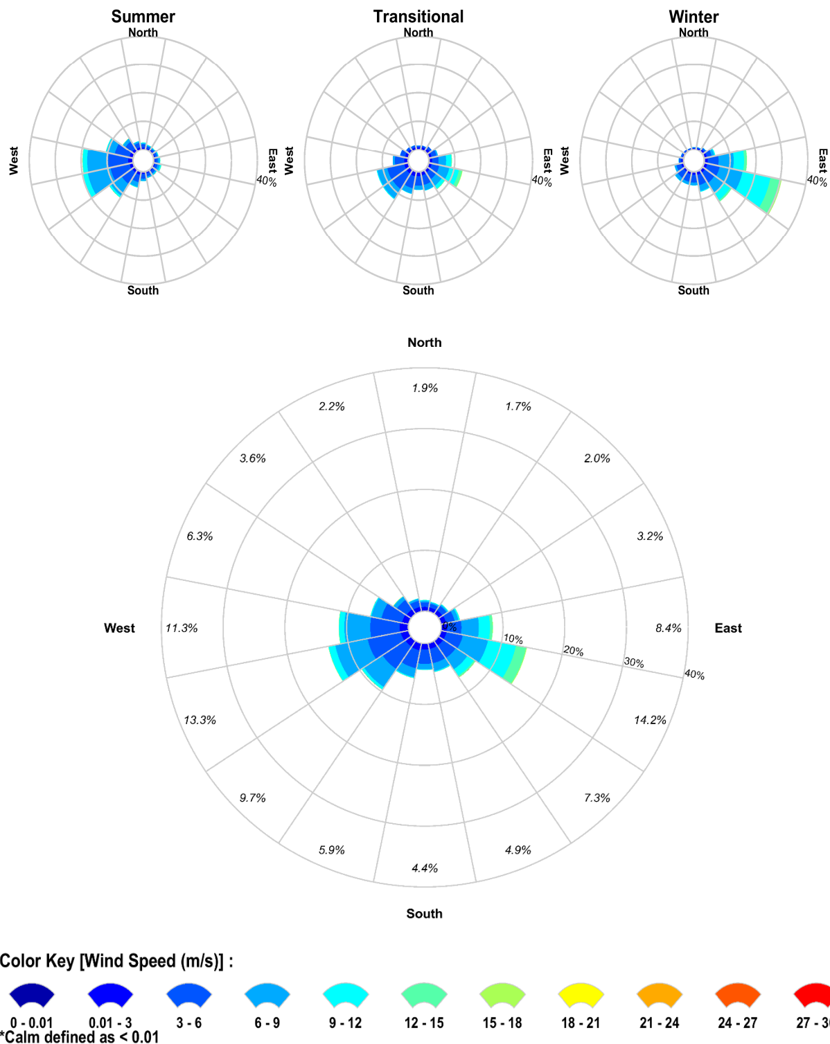
Figure 4.2 Seasonal (top) and total (bottom) wind distribution (2009-2018, inclusive) derived from the CFSR closest data point to the release locations. The colour key shows the wind magnitude, the compass direction provides the direction from which the wind is blowing, and the size of the wedge gives the percentage of the record.
