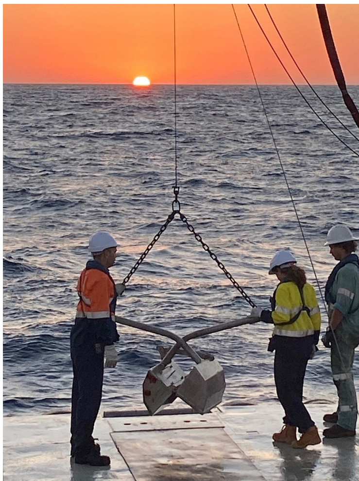
Plate 2-1: Deployment of van Veen grab sampler
