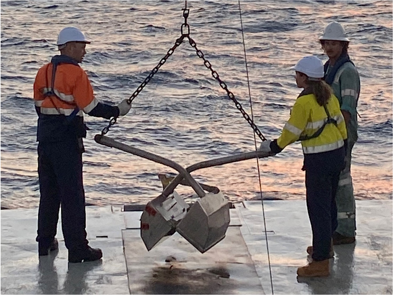
Figure 2-2: van Veen grab sampler being deployed during the study
