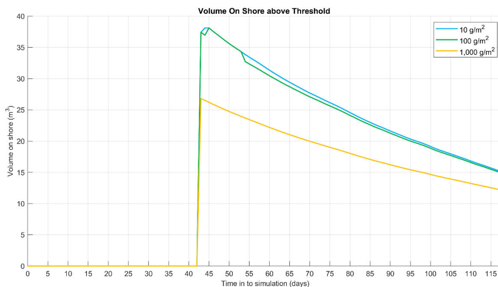
Figure 9.33 Time series of the volume on shore at the low (10-100 \text{g/m}^2 ), moderate (100-1,000 \text{g/m}^2 ) and high ( \geq 1,000 \text{ g/m}^2 ) thresholds for the simulation with the largest volume of oil ashore. Results are based on a surface blowout over 14 weeks, releasing a total 12,779,600 bbl (2,031,794 \text{m}^3 ) of crude from the WHP, tracked for 118 days, 6 am on the 24 th of February 2018.
