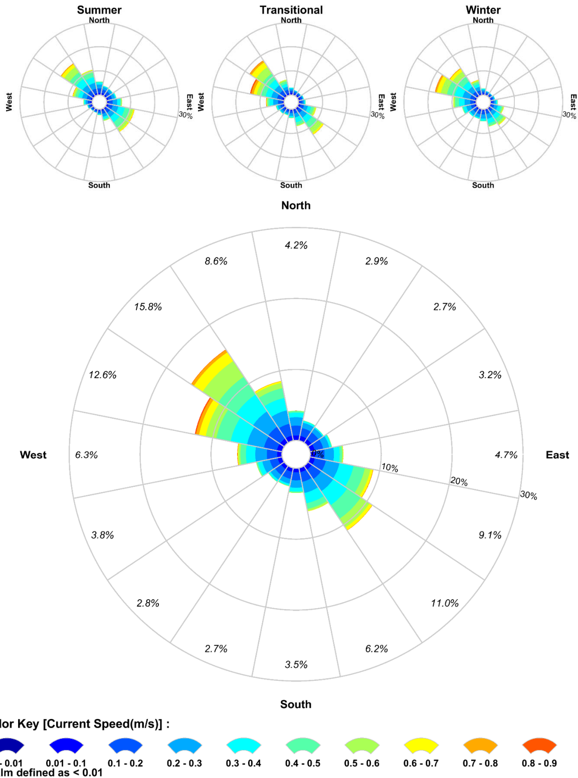
Figure 2.11 Seasonal (top) and total (bottom) current distribution (2009-2018, inclusive) derived from the HYCOM database near the Dorado Development area. The colour key shows the current magnitude, the compass direction provides the direction towards which the current is flowing, and the size of the wedge gives the percentage of the record.
