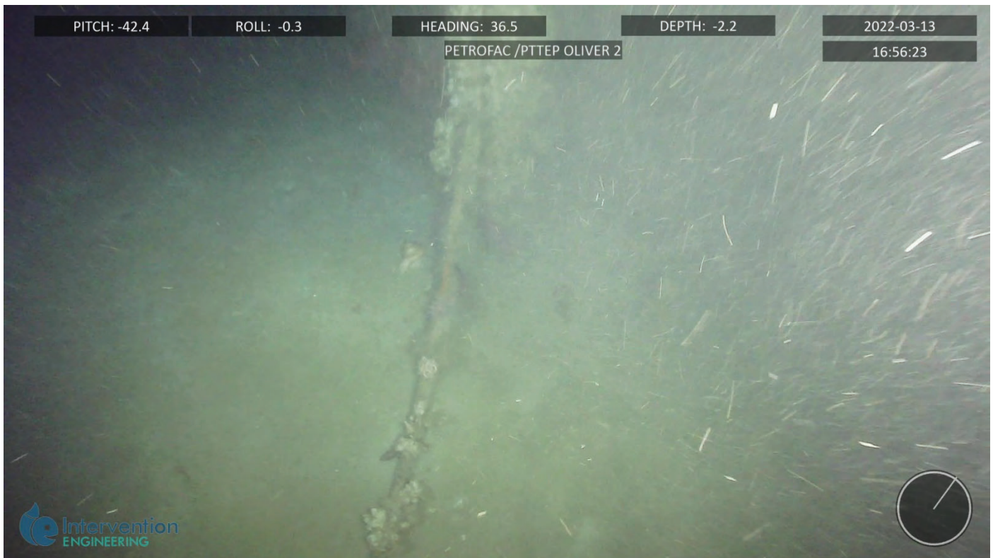
Figure 15 Oliver 2 Guide wire remenant in contact with seabed
