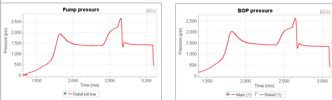
Figure 5. SLB Kill modelling, displacement of flowline
