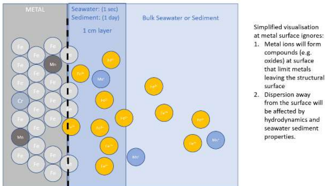
Figure 8-76 Schematic illustration of model used to derive element concentration at the steel surface in seawater and sediment
