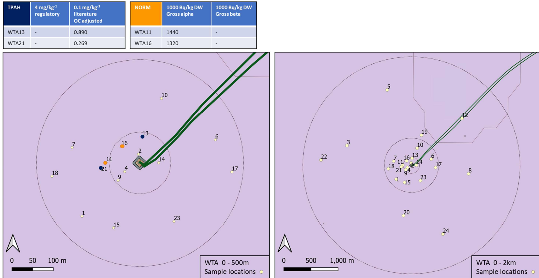
Figure 5-12 Sediment sampling locations around WTA platform.
