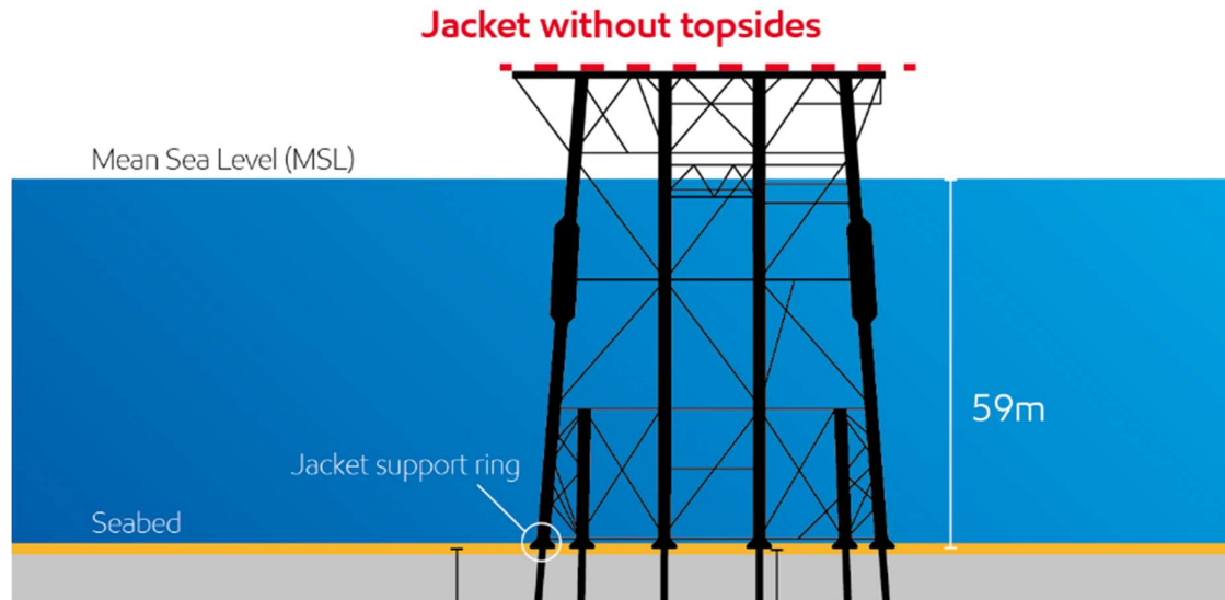
Figure 3-5 Schematic of Bream A facility showing indicative jacket support rings
