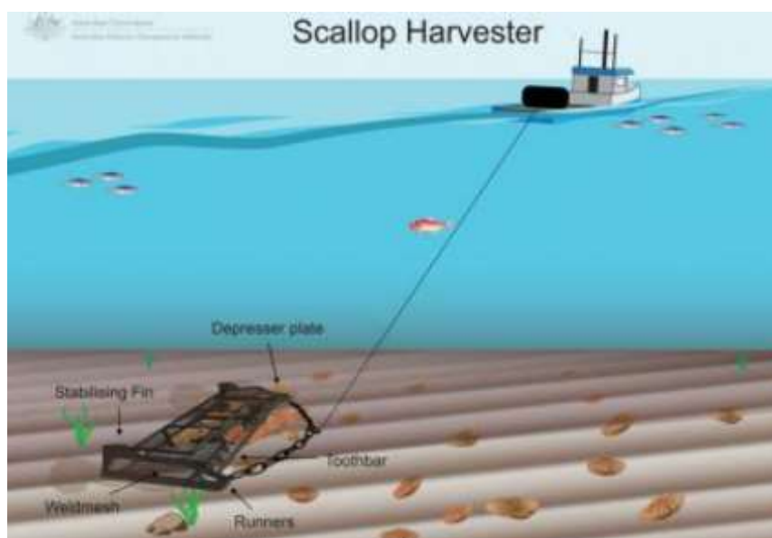
Figure 8-3 Scallop dredge main gear components
