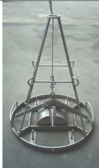
Figure M.9.1 Example of Spring-loaded Grab Sampler (Photo: Cawthron Inst.)
