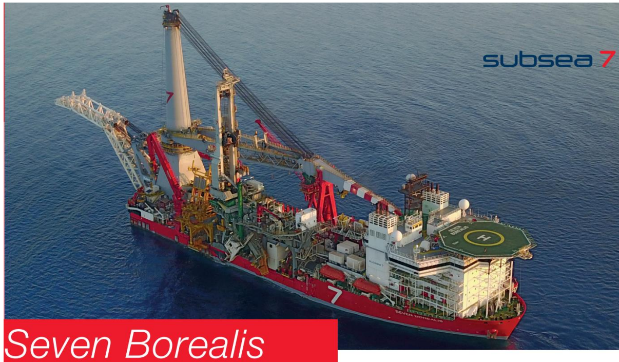
Figure 6. Subsea 7 Seven Borealis , the representative OCV and pipelay vessel.
