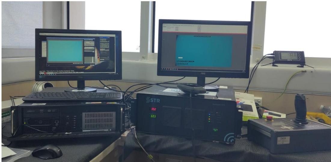
Figure 3: Topside unit controls for the SeaSpyder camera
