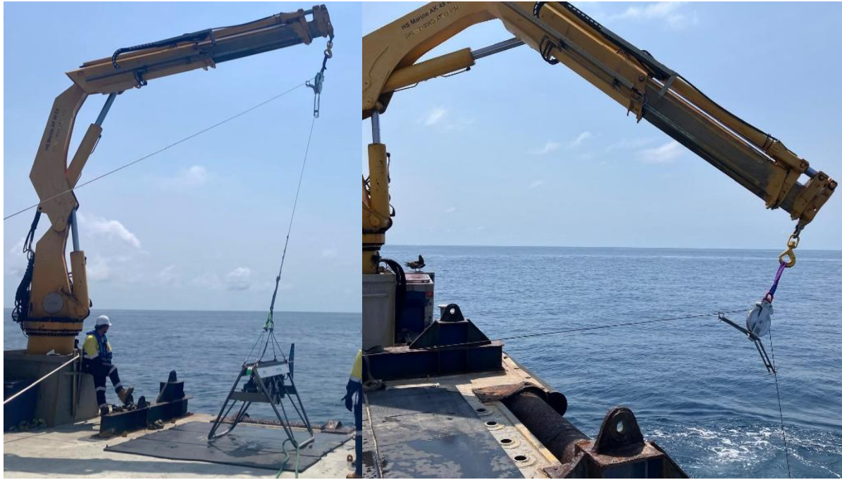
Figure 4: Overview of the set up for lifting operations (left) and during camera deployment (right)
