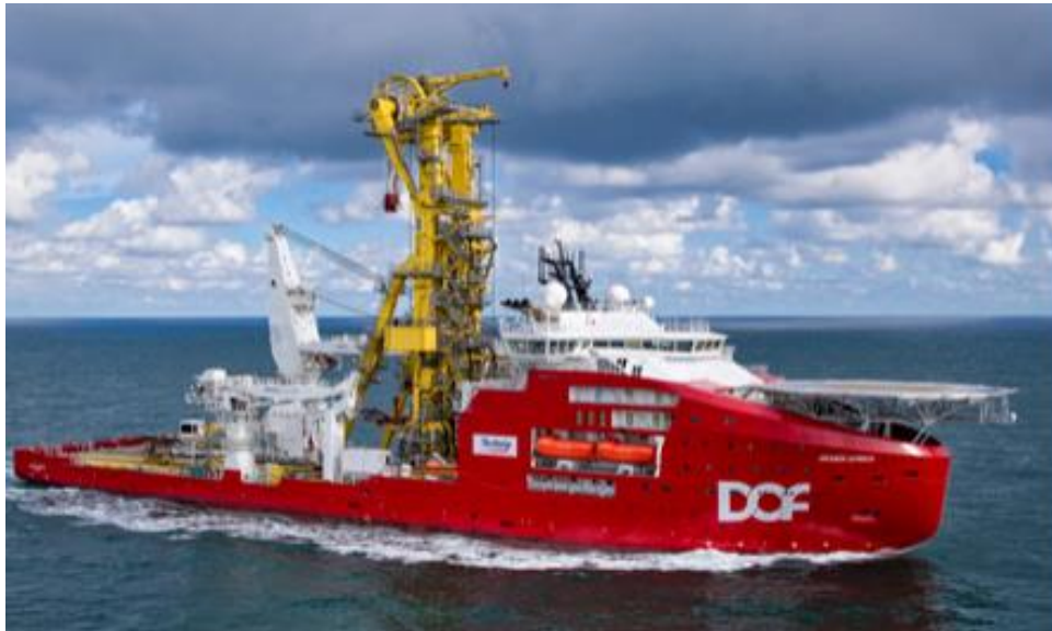
Figure 7. Skandi Africa , the representative pipelay construction support vessel.
