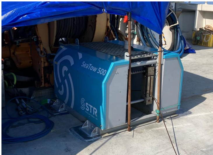
Figure 4: STR SeaTow 500 electric winch as set up during the field survey
